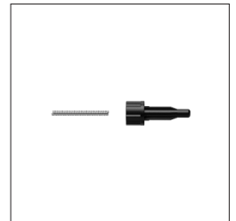
Remove the metal tube from the inlet guide tube.
