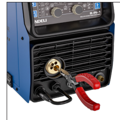
Remove the tube with long-nose pliers.
